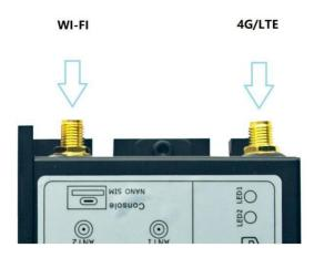
**NOTE:** The functions of the antennas are not fixed, maybe adjusted to cover other usage.
