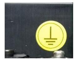
The PE signal is optional. If there is no EMI present, the PE connection can leave open.
