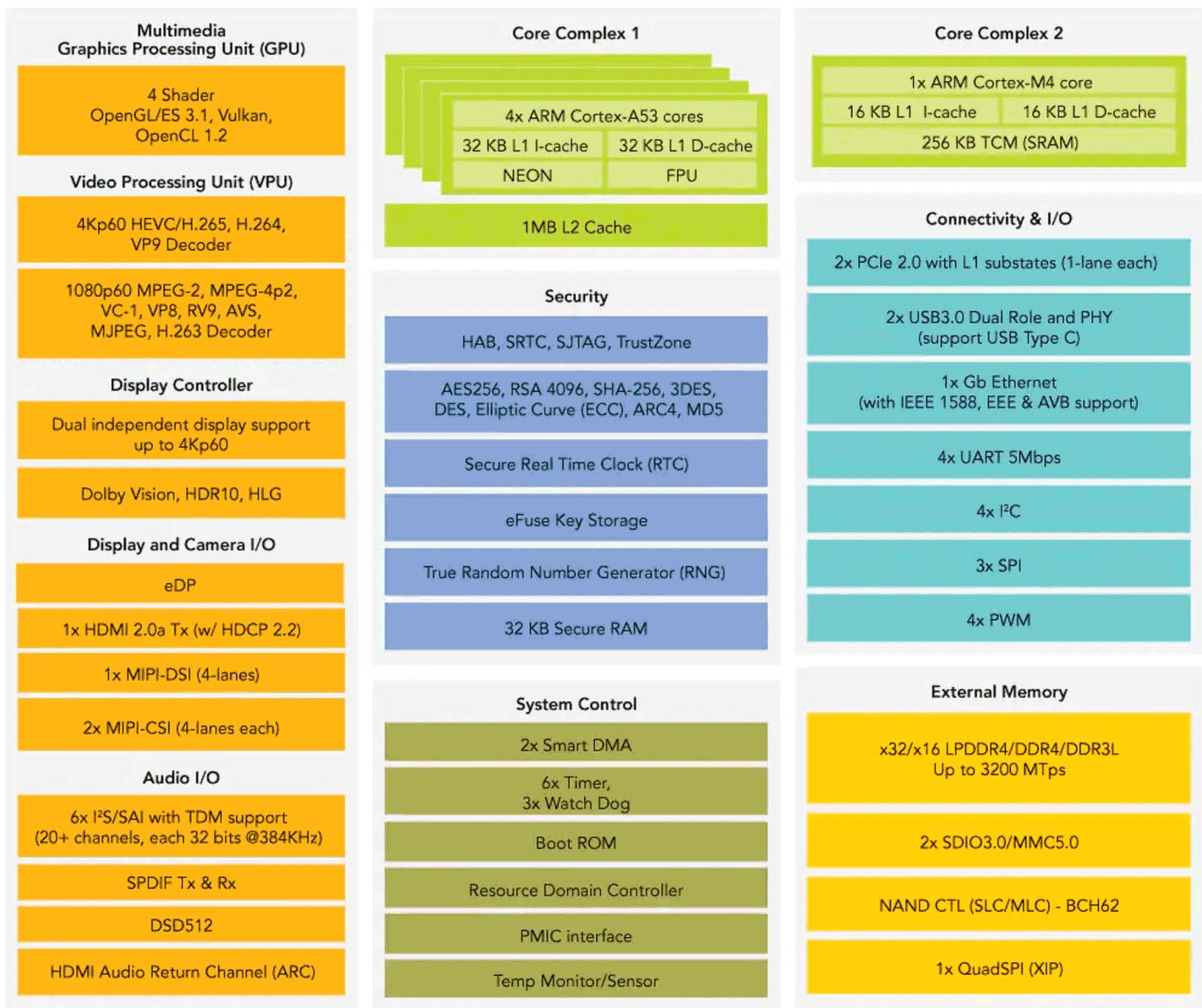
**Figure 2.** Block diagram of the i.MX8M SoC components, provided by NXP (some I/O signals on the SoC are consumed on the SoM, so refer to [table 1](#) for availability)
