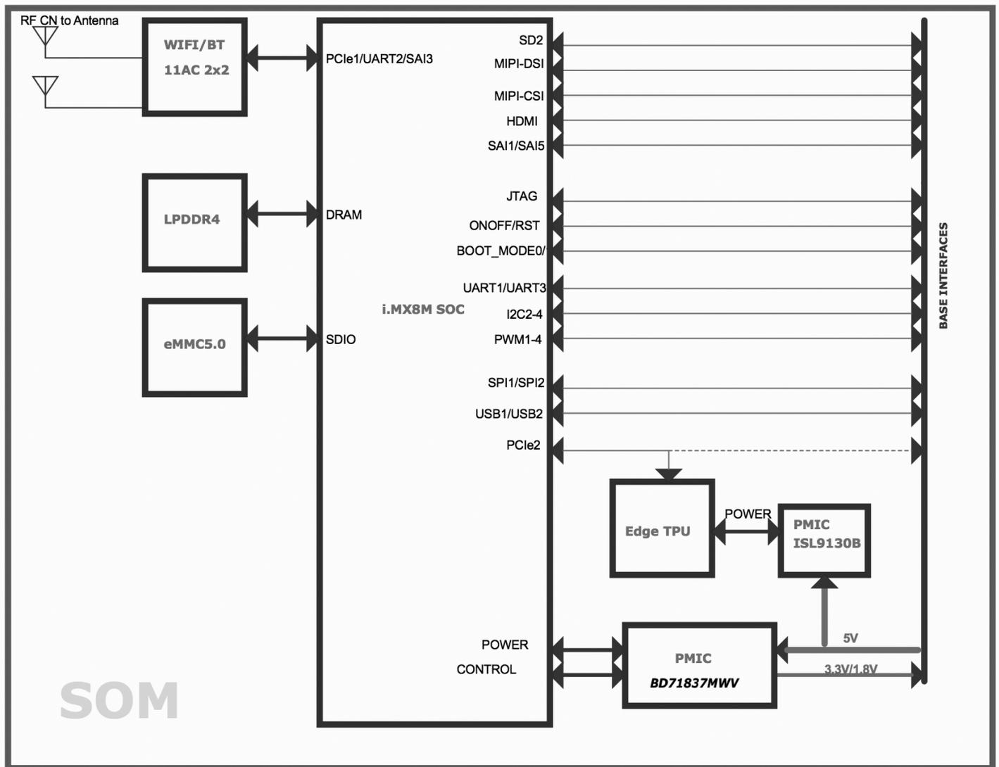
Figure 1. Block diagram of the SoM components
