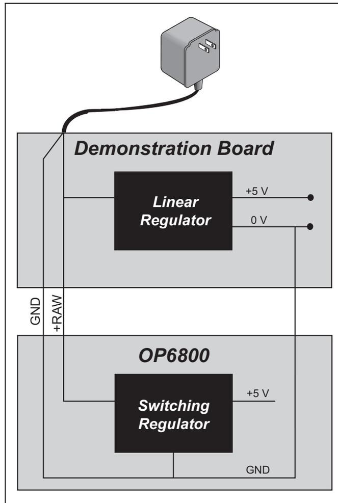
**Figure C-2. Power Distribution to OP6800 and Demonstration Board**
