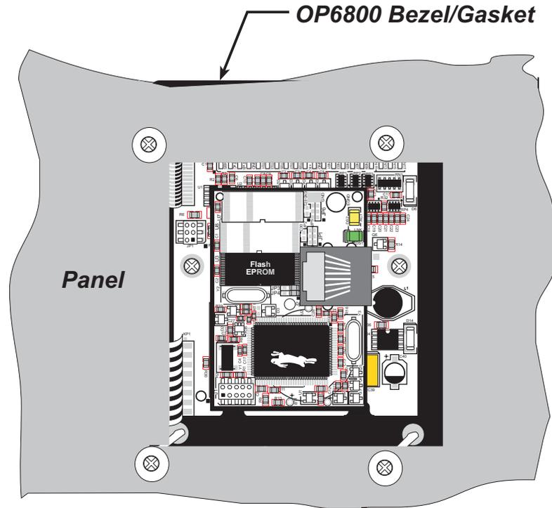
**Figure 21. OP6800 Mounted in Panel (rear view)**
