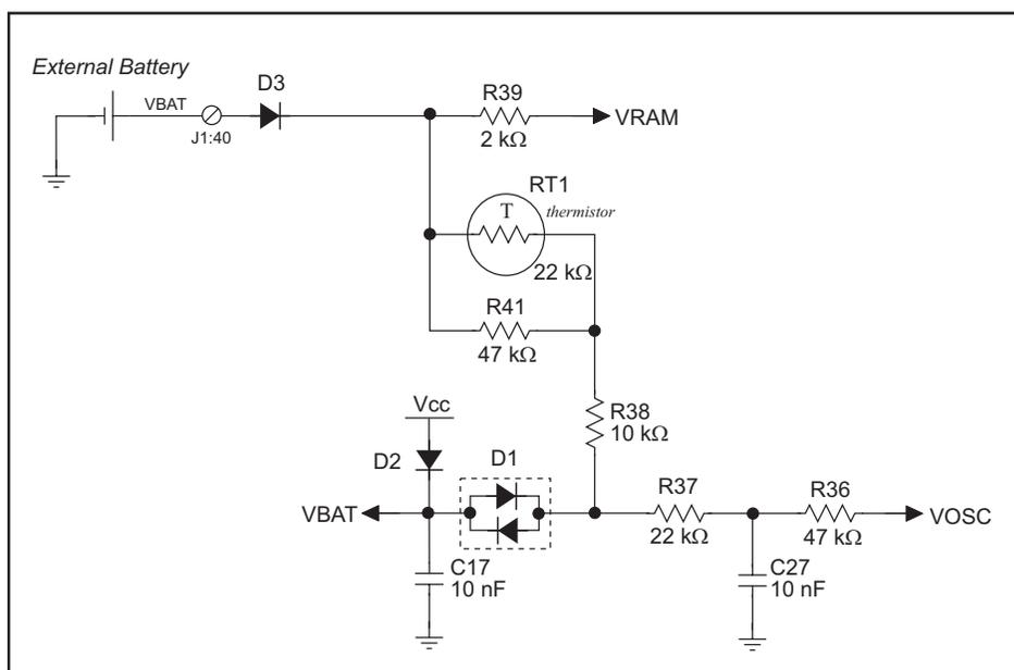
**Figure B-1. OP6800 Backup Battery Circuit**
