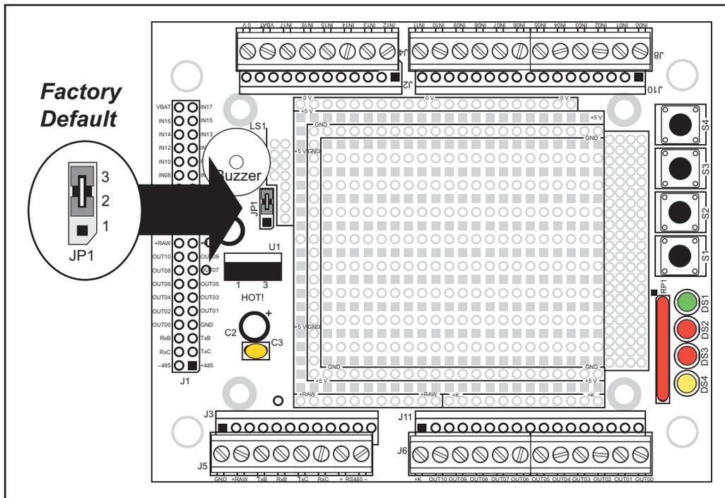
**Figure C-4. Demonstration Board Header JP1
