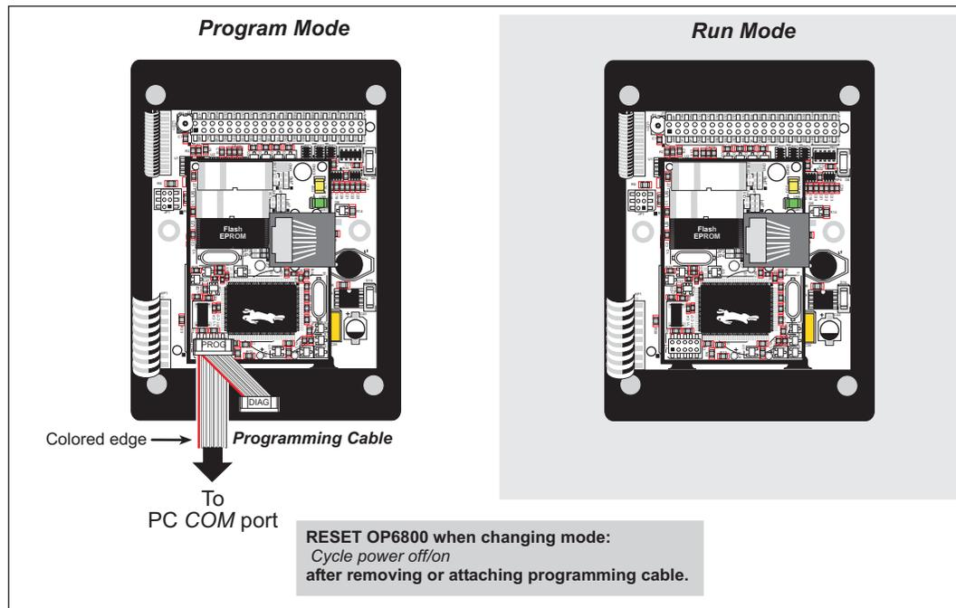
**Figure 15. OP6800 Program Mode and Run Mode Set-Up**
