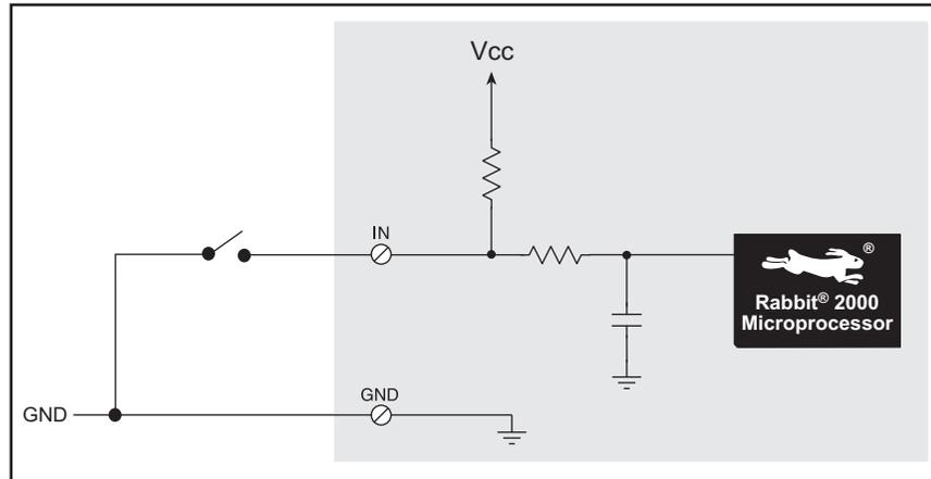
**Figure 9. OP6800 Digital Inputs**
