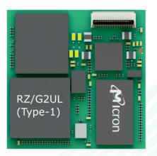
The Renesas G2UL or A3UL or FIVE SoC based LGA modules are designed as per the Open Standard Module<sup>TM</sup> Size-S Specification (OSM). This module can be integrated with any one of the three Renesas SoCs – G2UI, R3UL or FIVS SoCs. The FIVE SoC is based on RISC architecture (1 x RISC-V AX45MP) while the other two are ARM (1 x Arm® Cortex®-A55) based SoCs.
