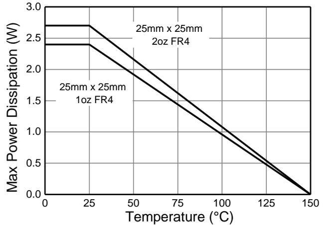
**Figure 2. Derating Curve**
