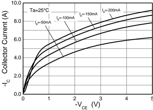
**Figure 6.  $I_C \text{ v } V_{CE}$**
