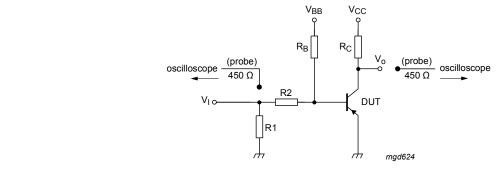
Fig. 13. Test circuit for switching times
