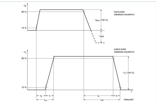
Fig. 12. BISS transistor switching time definition
