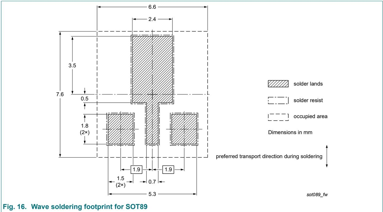
Fig. 16. Wave soldering footprint for SOT89
