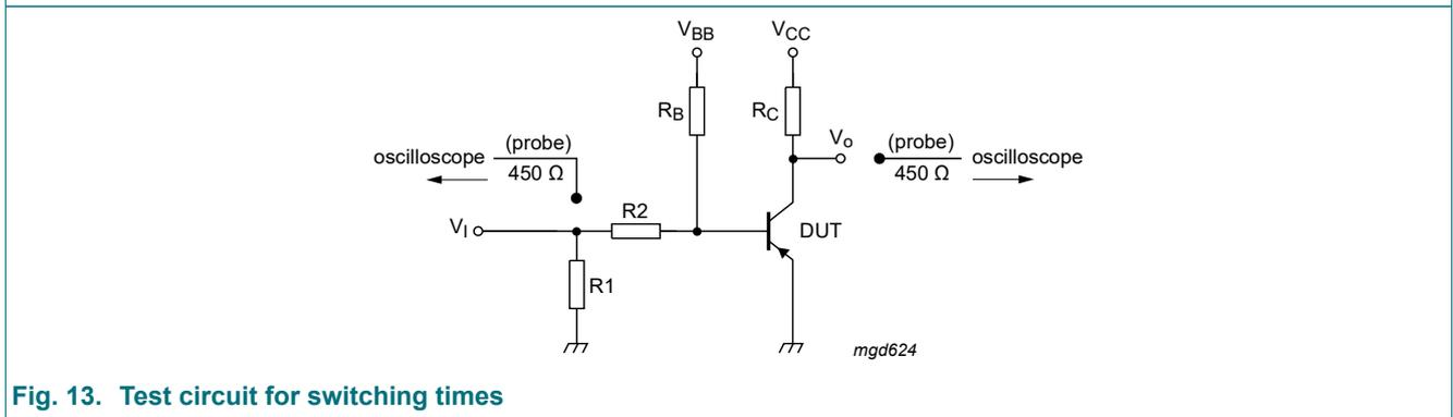
Fig. 13. Test circuit for switching times
