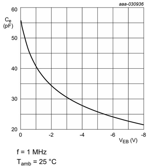
Fig. 27. BC806-25H-Q: Emitter capacitance as a function of emitter-base voltage; typical values
