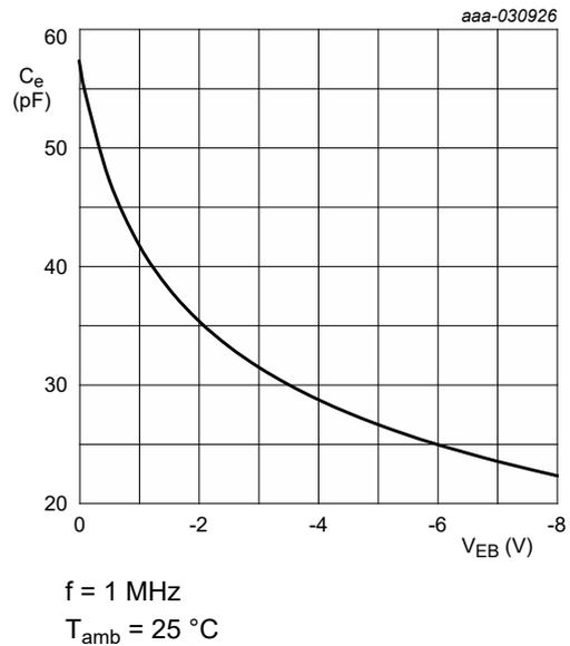
Fig. 15. BC806-16H-Q: Emitter capacitance as a function of emitter-base voltage; typical values
