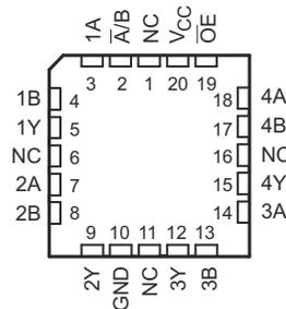
**Figure 4-3. FK Package, 20-Pin LCCC Top View**
