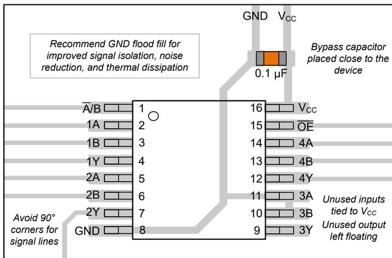
Figure 8-4. Example Layout for the SN74LVC257A
