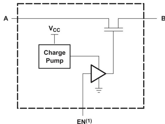
(1) EN is the internal enable signal applied to the switch.
