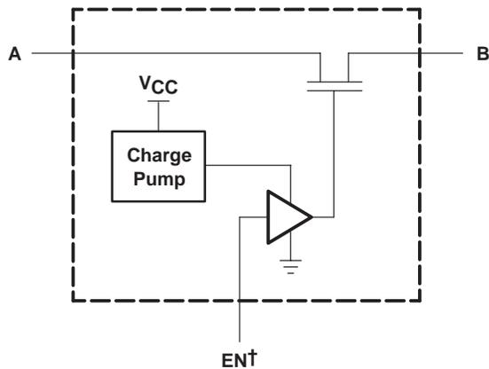
† EN is the internal enable signal applied to the switch.
