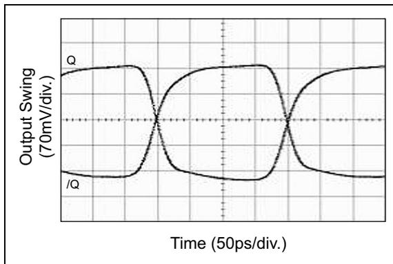
**FIGURE 2-2:** 2.5 GHz Output.
