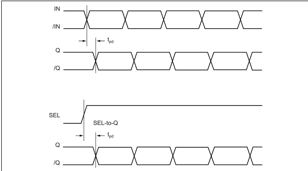
**FIGURE 4-1:** Timing Diagram.
