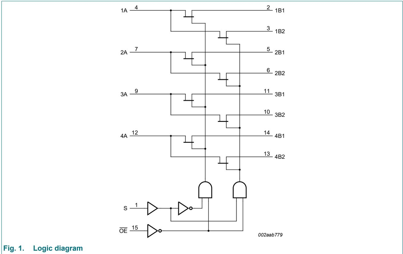
Fig. 1. Logic diagram
