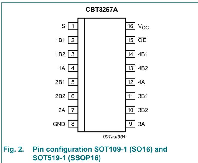
Fig. 2. Pin configuration SOT109-1 (SO16) and SOT519-1 (SSOP16)
