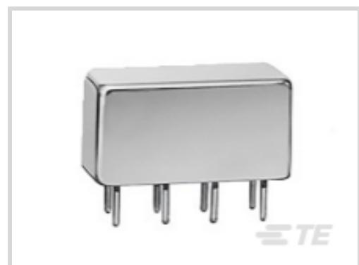
Contact Arrangement: **2 Form C, DPDT, 2 C/O**Input Voltage: **12 VDC**Contact Current Rating: **2 A**Coil Voltage Rating: **12 VDC**Coil Resistance: **160 Ω**
