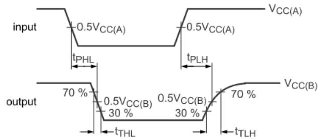
**Figure 3: Propagation Delay and Transition Times A→B**
