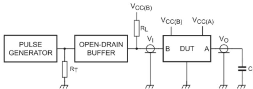
$R_L$  = load resistor; 1.35 k $\Omega$  on port B
