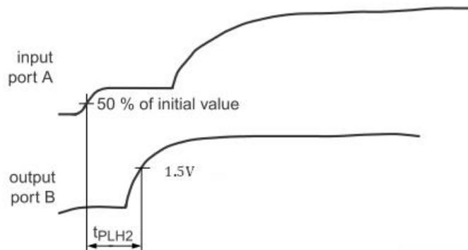
**Figure 4: Propagation delay from the port A's external driver switching off to port B LOW-to-HIGH transition; (A→B)**
