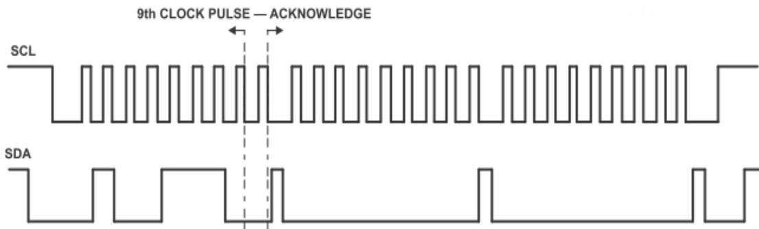
Figure 7: Bus B I<sup>2</sup>C/SMBus Waveform
