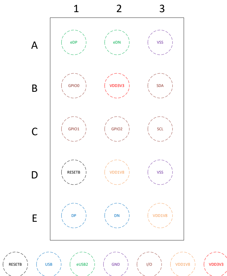
Figure 5-1. TUSB2E11 YCG Package, 15-Pin DSBGA (Top View)
