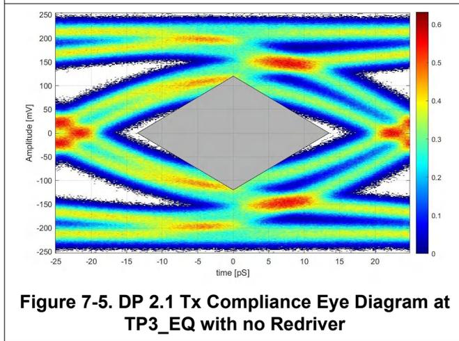
**Figure 7-5. DP 2.1 Tx Compliance Eye Diagram at TP3\_EQ with no Redriver**
