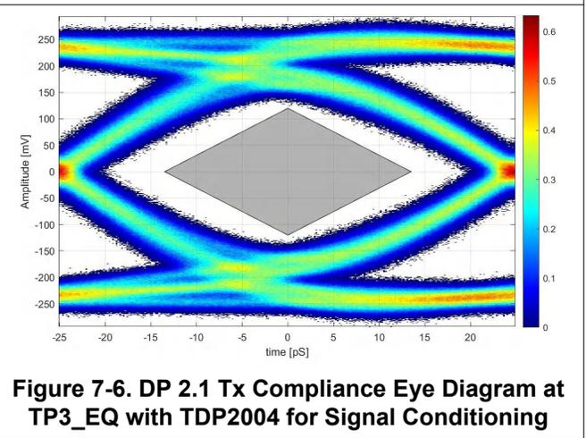
**Figure 7-6. DP 2.1 Tx Compliance Eye Diagram at TP3\_EQ with TDP2004 for Signal Conditioning**
