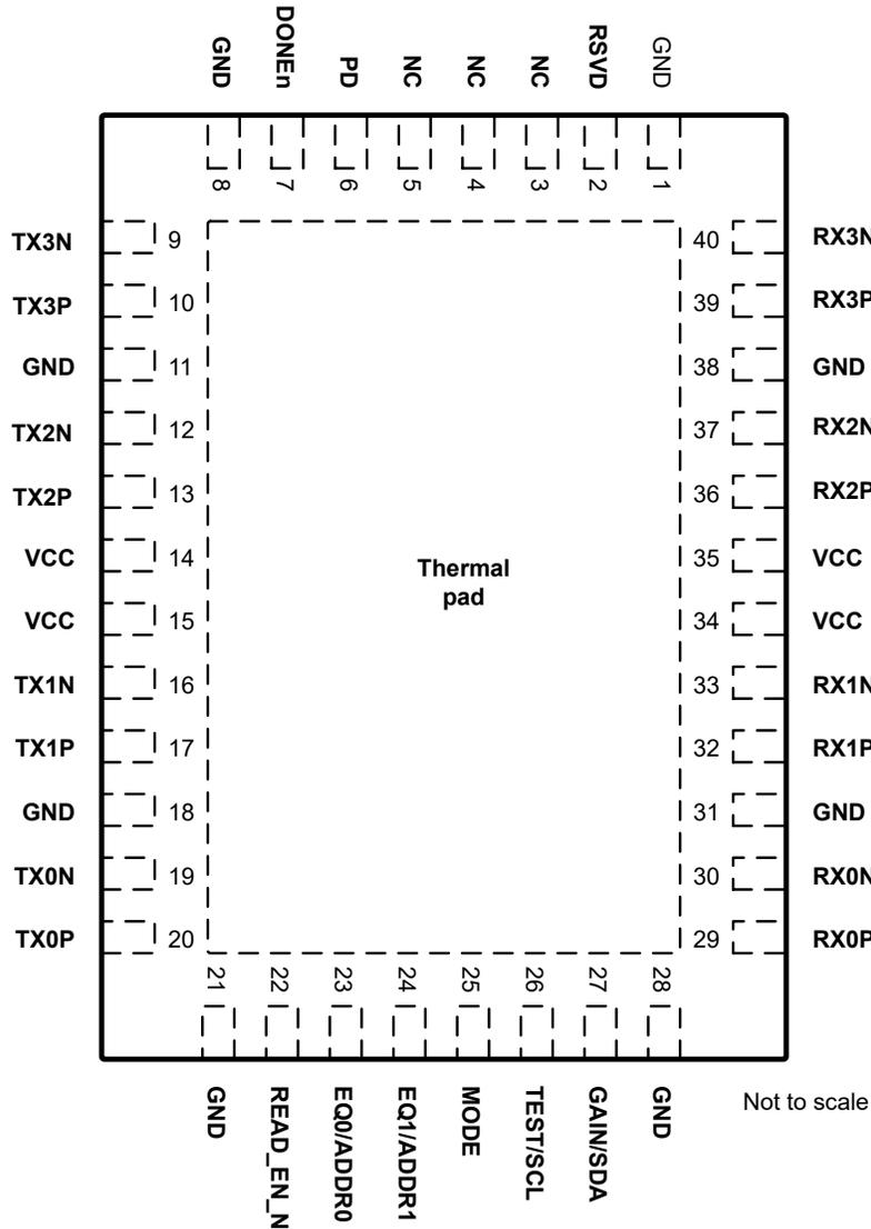
Figure 4-1. RNQ Package, 40-Pin WQFN (Top View)
