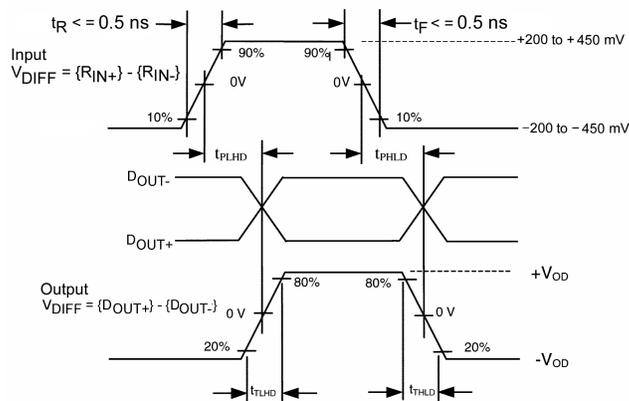
FIGURE 4. AC Waveform
