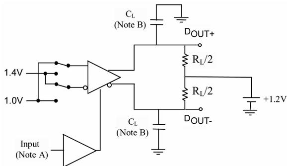
Note A: All LVTTTL input pulses have frequency = 10MHz,  $t_R$  or  $t_F$  <= 2 ns
