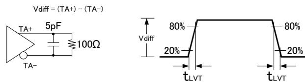
Figure 5. LVDS Output Load and Transition Time
