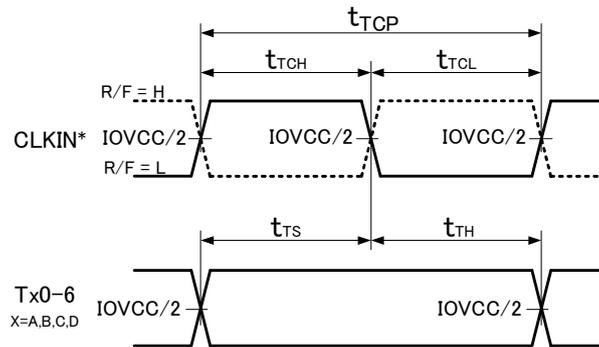
**Figure 4. CLKIN and Tx0-6 Input Timings**
