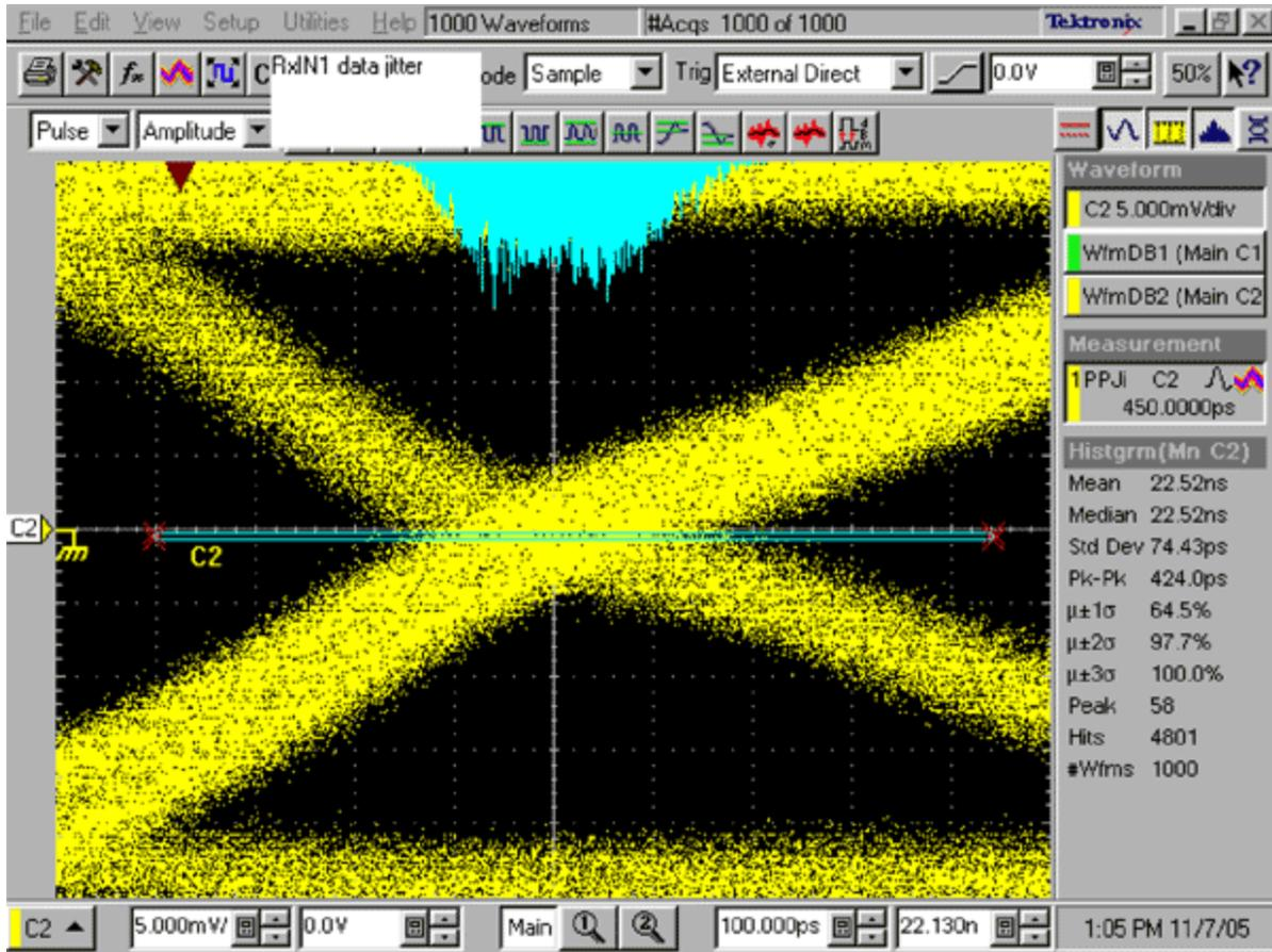
Figure 3. Data jitter measurement.
