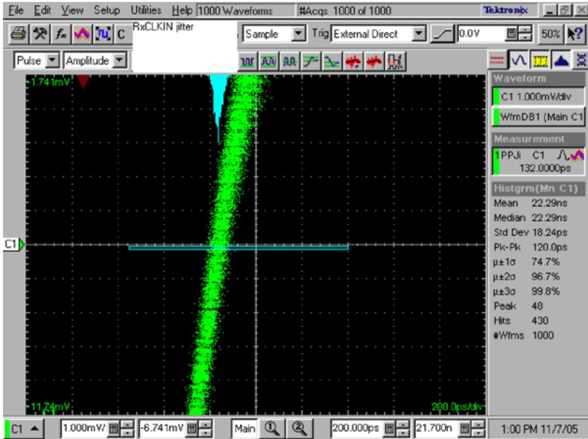
Figure 1. Clock jitter measurement at 0V differential.
