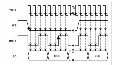
Figure 1. Sampling of I<sup>2</sup>S input signals.
