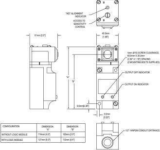
Figure 19. Dimensions for the fiber models
