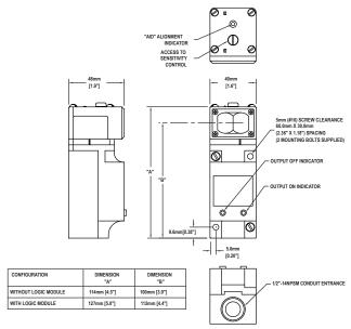
Figure 18. Dimensions for the FF models
