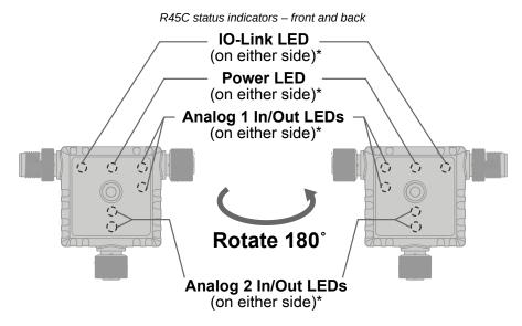
\* Indicator LEDs are visible through translucent housing
