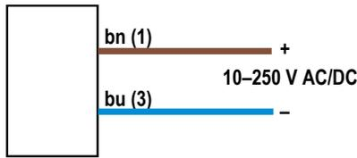
Figure 2. Emitters - QD (3-Pin 7/8 in-16UNF )
