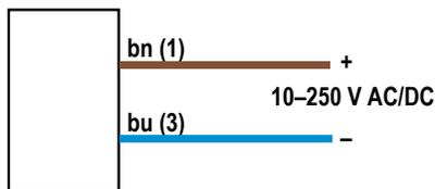
Figure 8. Emitters - QD (3-Pin 7/8 in-16UNF )
