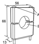
Hole center spacing: A=ø 45
