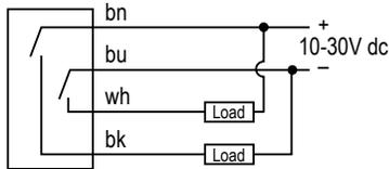
Figure 5. Other DC Models - QD (4-Pin 7/8 in-16UNF )
