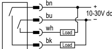
Figure 6. 4-Pin 7/8 in-16UNF Pinout
