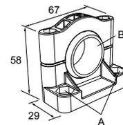
Hole center spacing: A=ø 50.8
