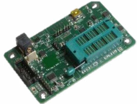
There are three different types of Linear Array demo kits. The simplest is USEQDAK6000000, a microprocessor powered board which interfaces to a PC and allows the user to test and evaluate the linear arrays listed in the table. These supported sensors are not included in the kit.
