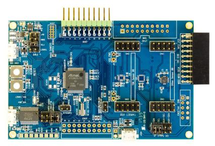
The development kit comes with necessary software including InvenSense MotionLink, a GUI based development tool and embedded Motion Drivers for ICM-20602.
