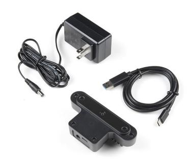
firmware, and software suite combine depth perception, object detection (neural inference), and object tracking and gives you this power in a simple, easy-to-use Python API. This Oak-D variant of DepthAI allows the power of the Myriad X VPU to be fully harnessed and used with the platform of your choice.
