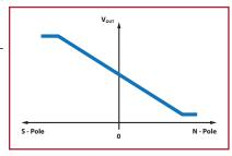
Applications: This sensor can be used to measure precise magnet linear or rotation position using the analog output.
