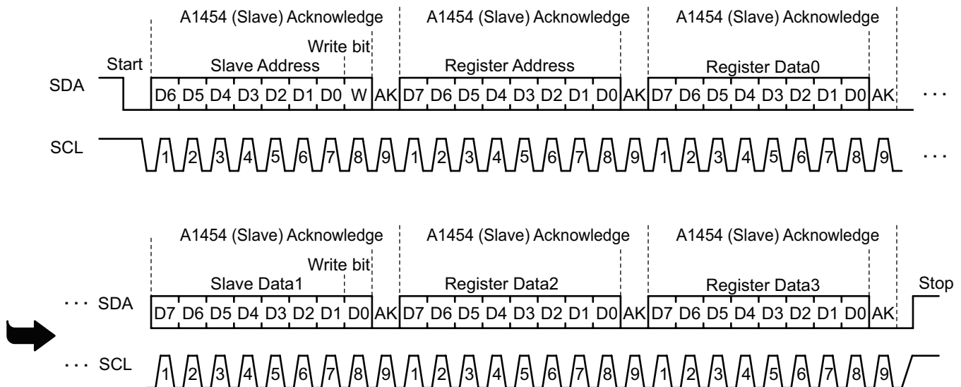
Figure 2: I 2 C Write Operation
