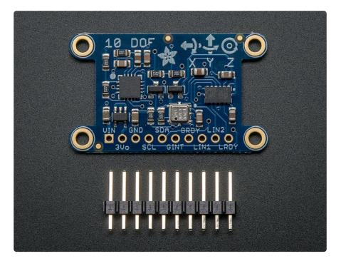
To interface with the sensor, you will need to solder in wire or header into the breakout row at the bottom. You cannot 'press fit' or 'twist' wires in, they will not make good contact! Soldering is required
