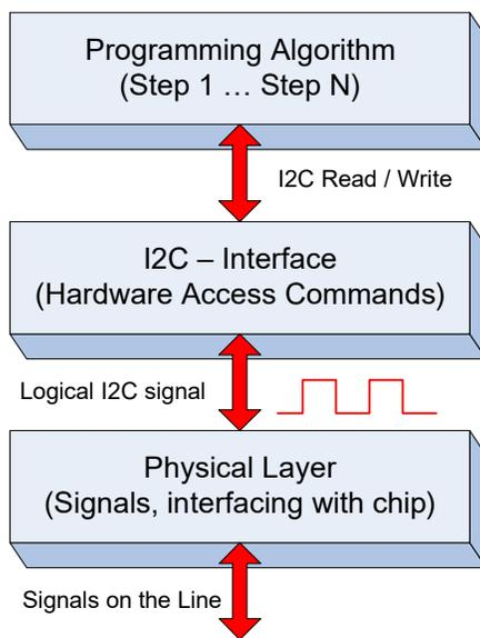
The Programming Algorithm protocol—the topmost protocol—implements the whole programming flow in terms of atomic I2C commands. It is the most solid and fundamental part of this specification. For more information on this algorithm, see [Chapter 4: Programming Algorithm](#).
