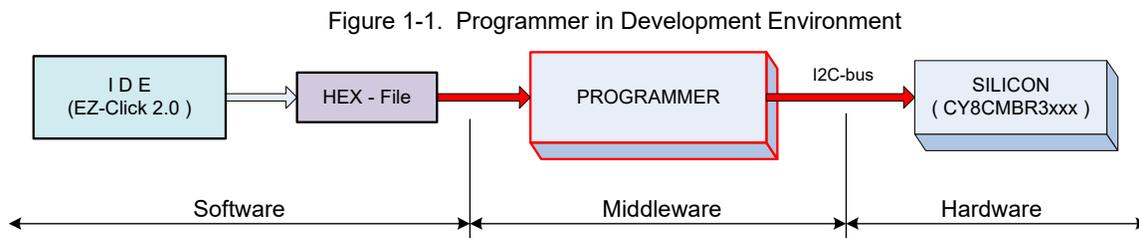
In the manufacturing environment, the IDE block is absent because its main purpose is to produce a hex file.
