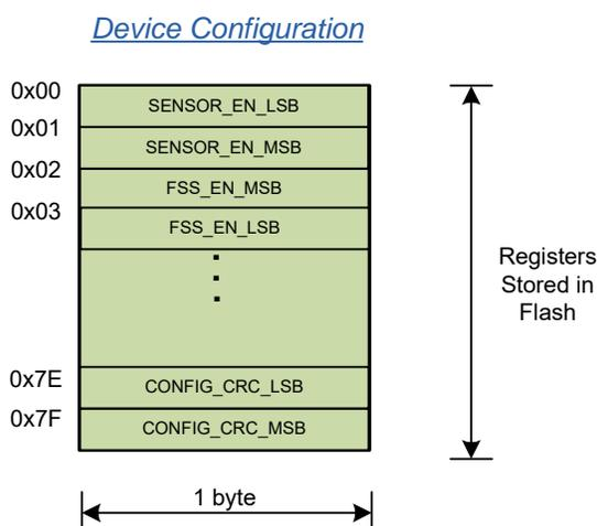
The flash memory is mapped directly to the I/O registers of the silicon; 128 bytes of flash configure 0x00-0x7F registers of the Device Configuration state. Programmer extracts all 128 bytes from the hex file.
