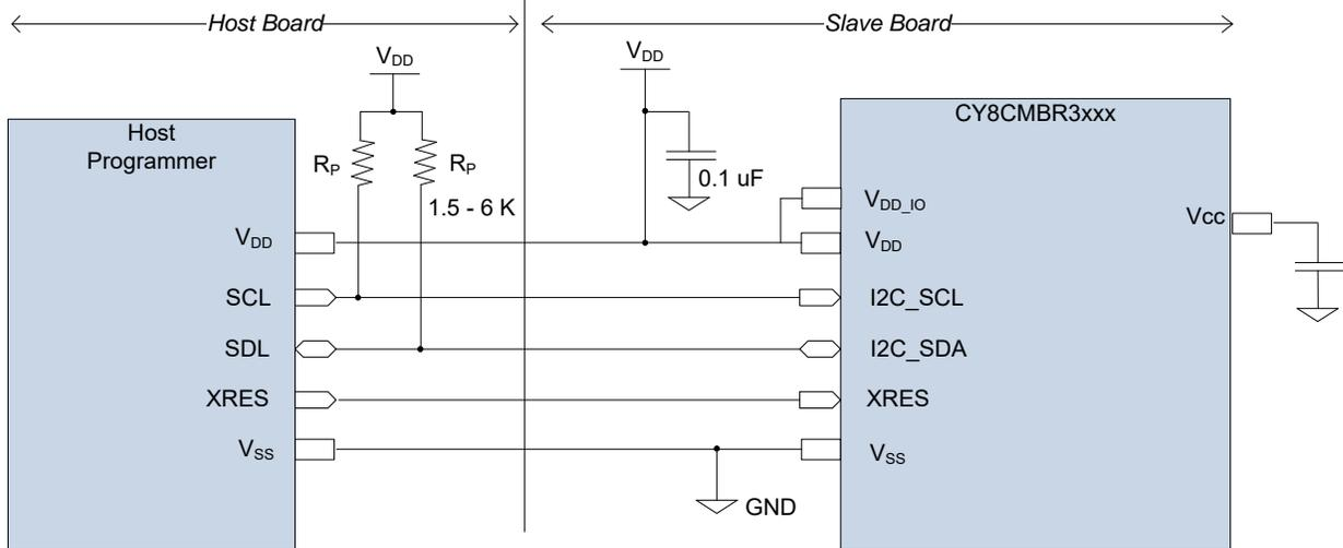
Note 1: The V<sub>DD\_IO</sub> supply is pin available only the selected packages. For the packages that have a V<sub>DD\_IO</sub> pin, the V<sub>DD</sub> and V<sub>DD\_IO</sub> pins should be connected together (shorted) on the board.
