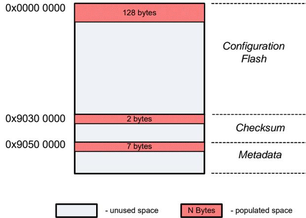
**0x0000 0000 - Configuration Data** (128 bytes), which must be programmed into the flash. These bytes configure the CY8CMBR3xxx device during boot.
