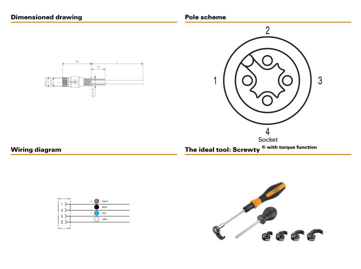
Light, securely screwed-in round plug-in connectors. Screwty set DM / VPE: 1 / Order No.: 192000000 Adapters: M12, M12 F, M8, M8 F
