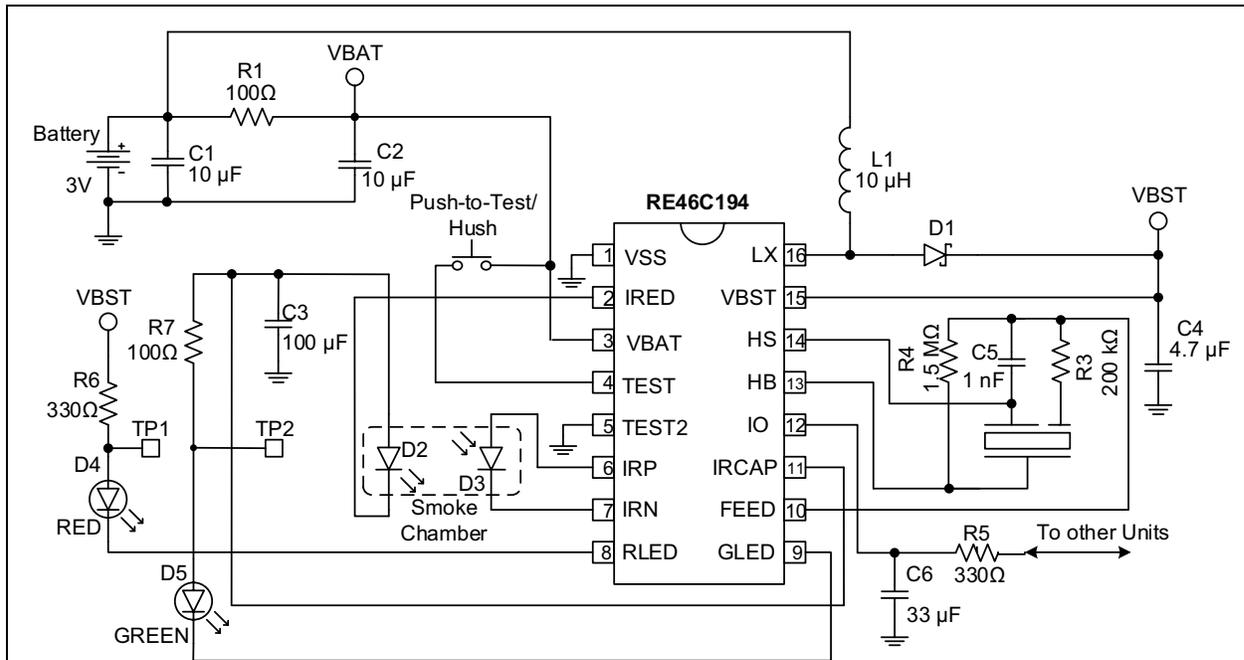
**Note 1:** C2 should be located as close as possible to the device power pins, and C1 should be located as close as possible to the VSS power input connection.
