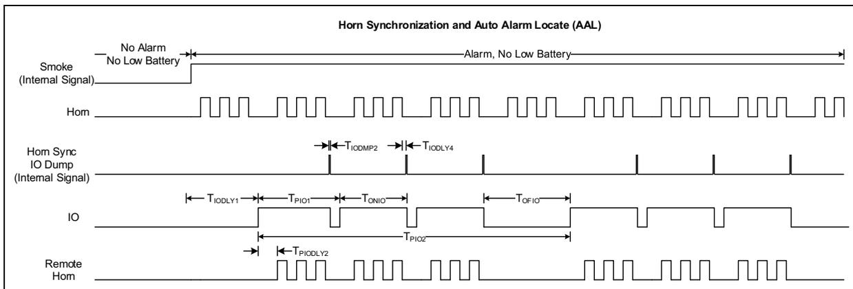
**FIGURE 5-5:** Timing Diagram - Horn Synchronization and AAL.
