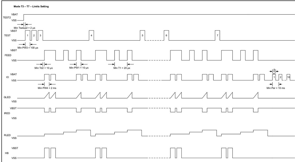
**FIGURE 4-6:** Timing Diagram for Modes T3 to T7.
