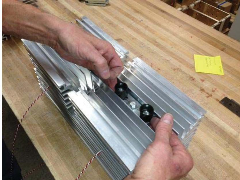
Fig. 5 - Step 3: Drop the clamp into the top heatsink
