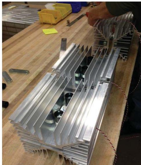
Fig. 8 - Step 6: Check to make sure the two mounting surfaces are still parallel. Tighten each bolt a 1/10<sup>th</sup> turn more. Do not tighten beyond this point.
