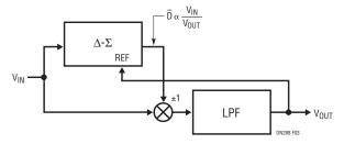
Figure 3. LTC1966 Block Diagram
