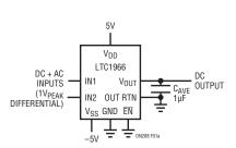
Figure 1a. ±5V Supplies, Differential, DC-Coupled RMS-to-DC Converter
