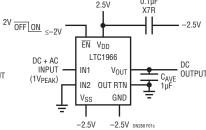
Figure 1c. ±2.5V Supplies, Single Ended, DC-Coupled RMS-to-DC Converter with Shutdown
