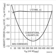
Figure 2. Quantum Leap in Linearity Performance
