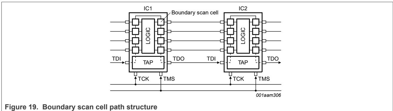
Figure 19. Boundary scan cell path structure
