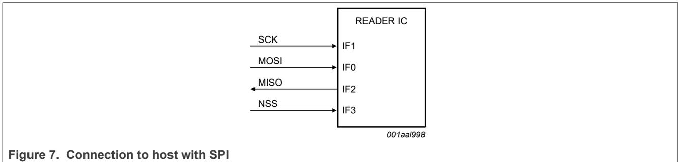
Figure 7. Connection to host with SPI
