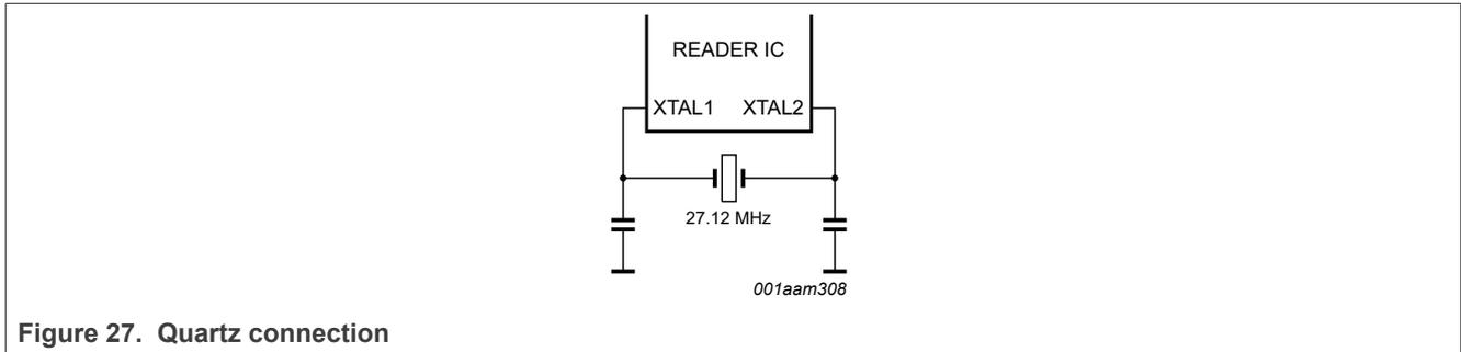
Figure 27. Quartz connection
