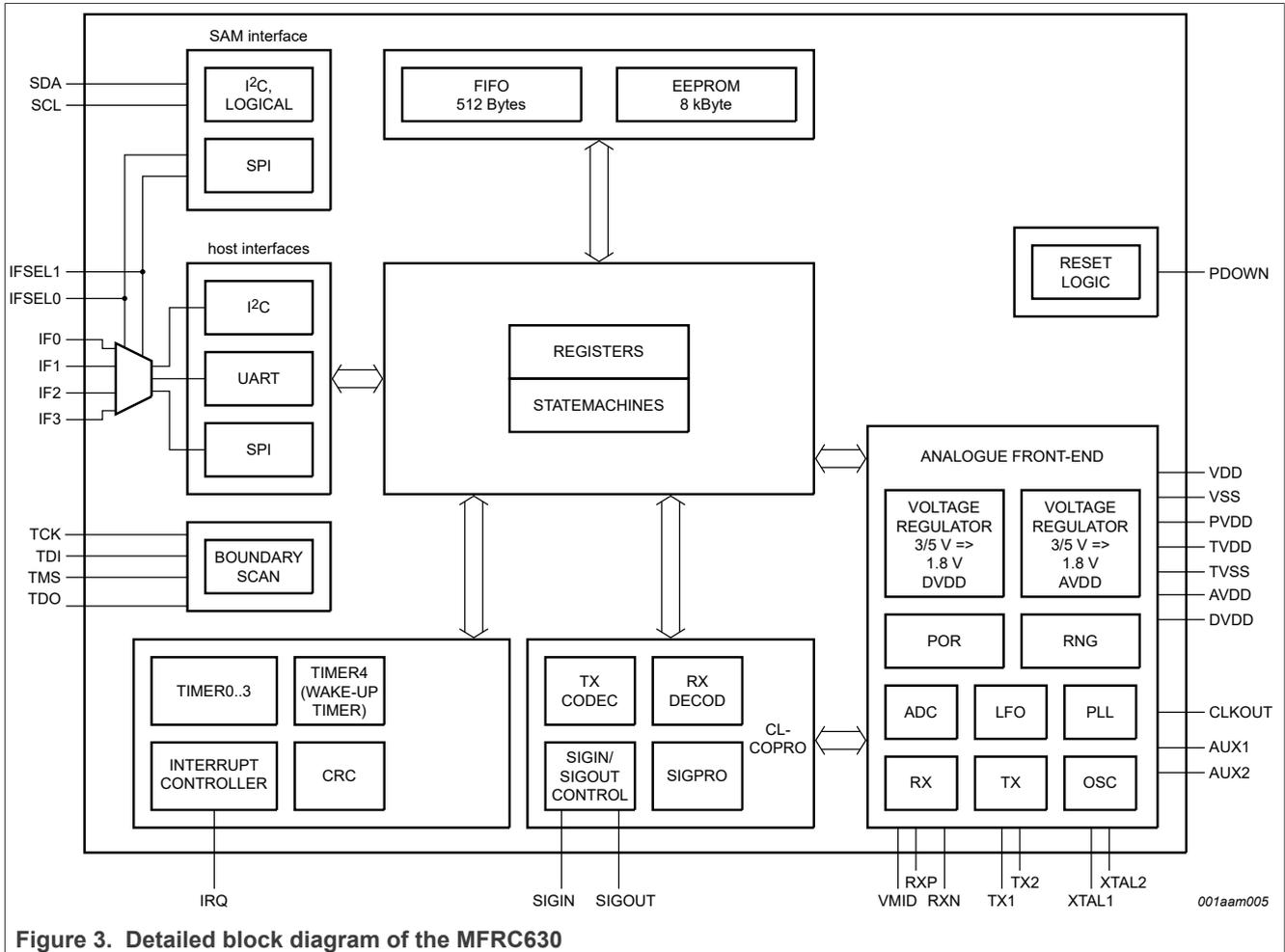
Figure 3. Detailed block diagram of the MFRC630
