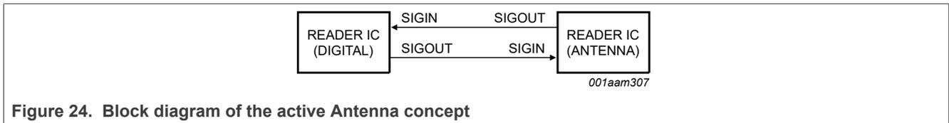
Figure 24. Block diagram of the active Antenna concept
