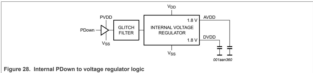
Figure 28. Internal PDown to voltage regulator logic
