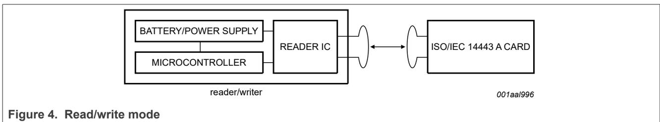
A typical system using the MFRC630 is using a microcontroller to implement the higher levels of the contactless communication protocol and a power supply (battery or external supply).
