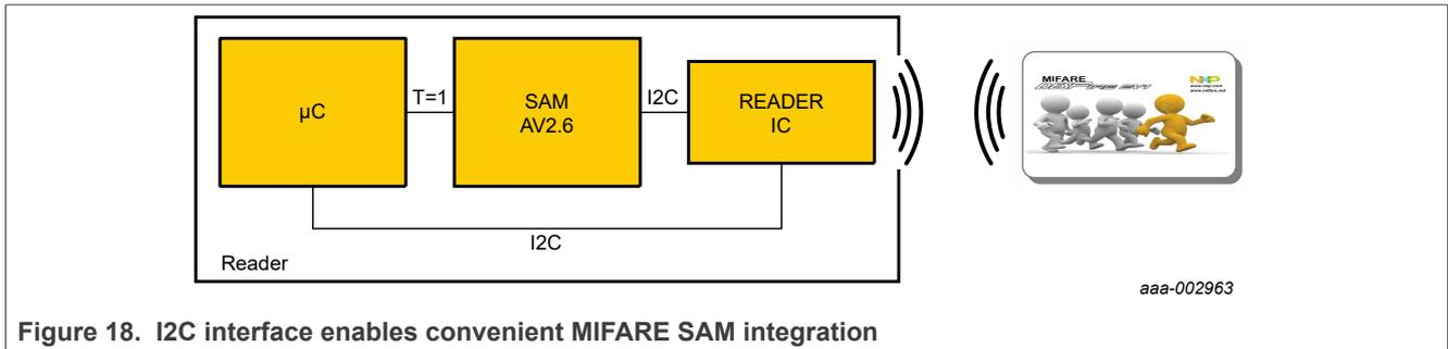
Figure 18. I2C interface enables convenient MIFARE SAM integration
