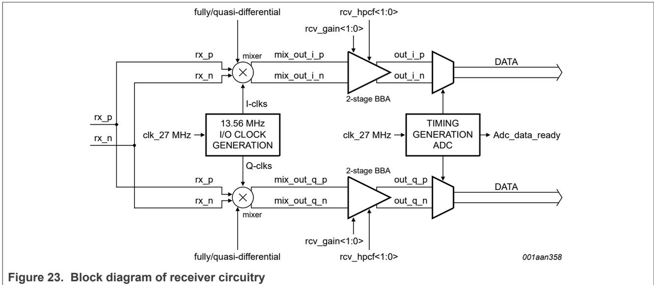
Figure 23. Block diagram of receiver circuitry
