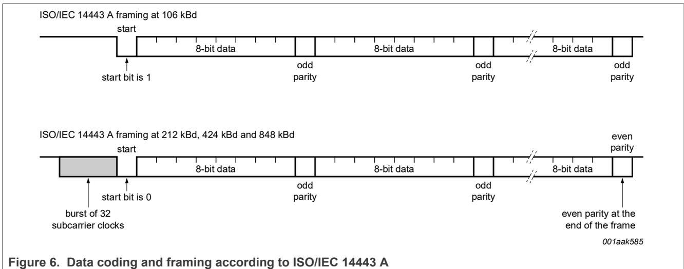
The internal CRC coprocessor calculates the CRC value based on ISO/IEC 14443 A part 3 and handles parity generation internally according to the transfer speed.
