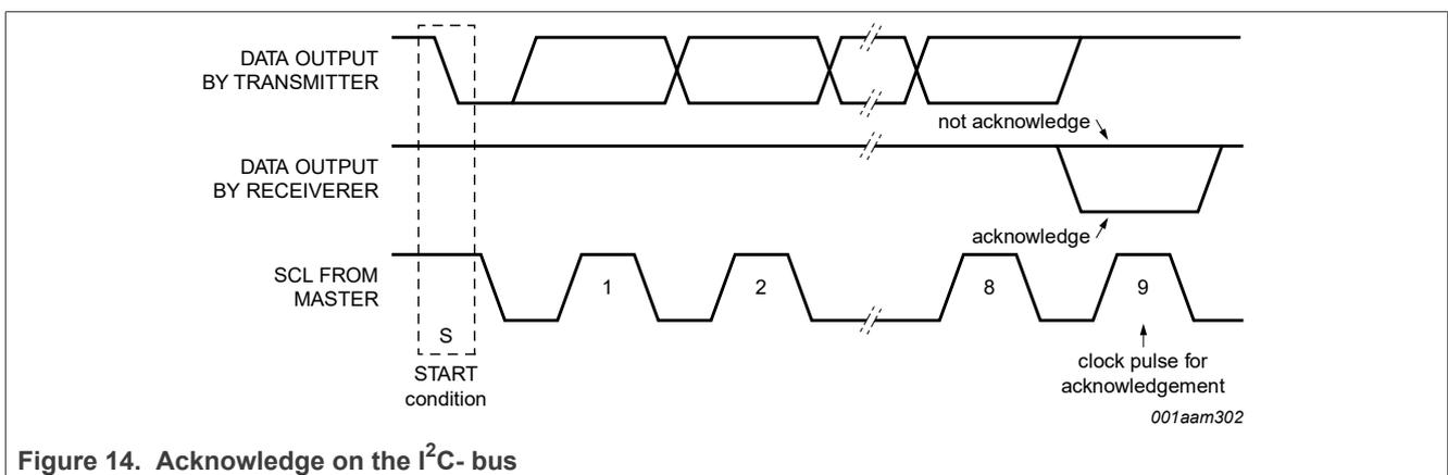
Figure 14. Acknowledge on the I<sup>2</sup>C- bus
