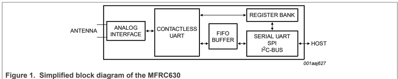
Figure 1. Simplified block diagram of the MFRC630
