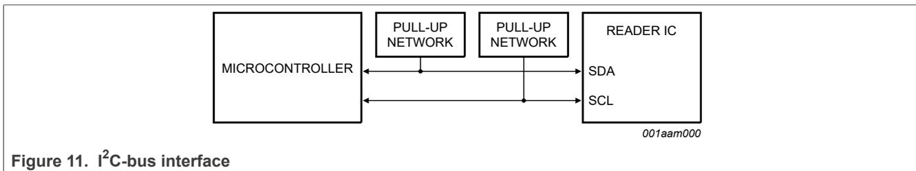
The voltage level on the I2C pins is not allowed to be higher than PVDD.
