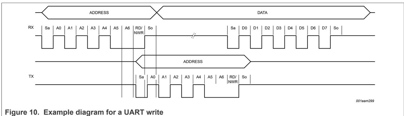
Figure 10. Example diagram for a UART write
