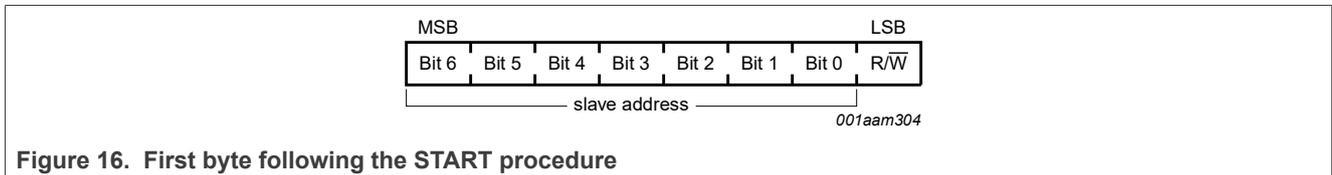
Figure 16. First byte following the START procedure
