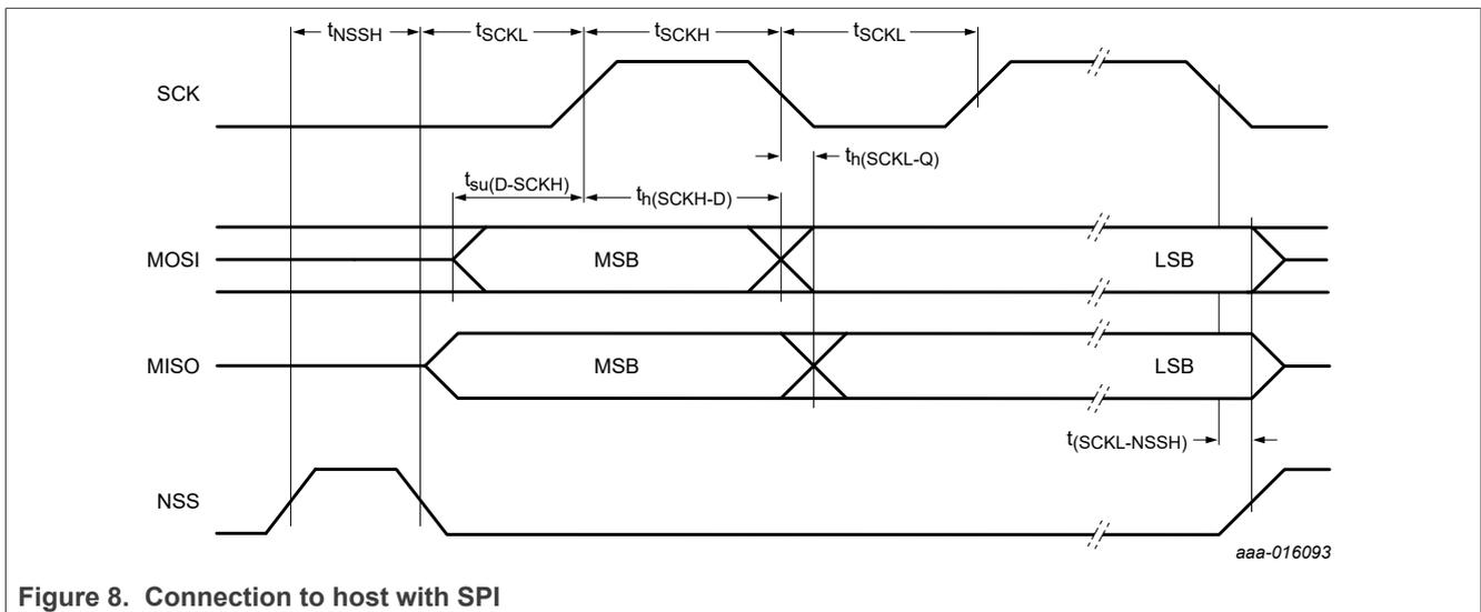
**Remark:** To send more bytes in one data stream the NSS signal must be LOW during the send process. To send more than one data stream the NSS signal must be HIGH between each data stream.
