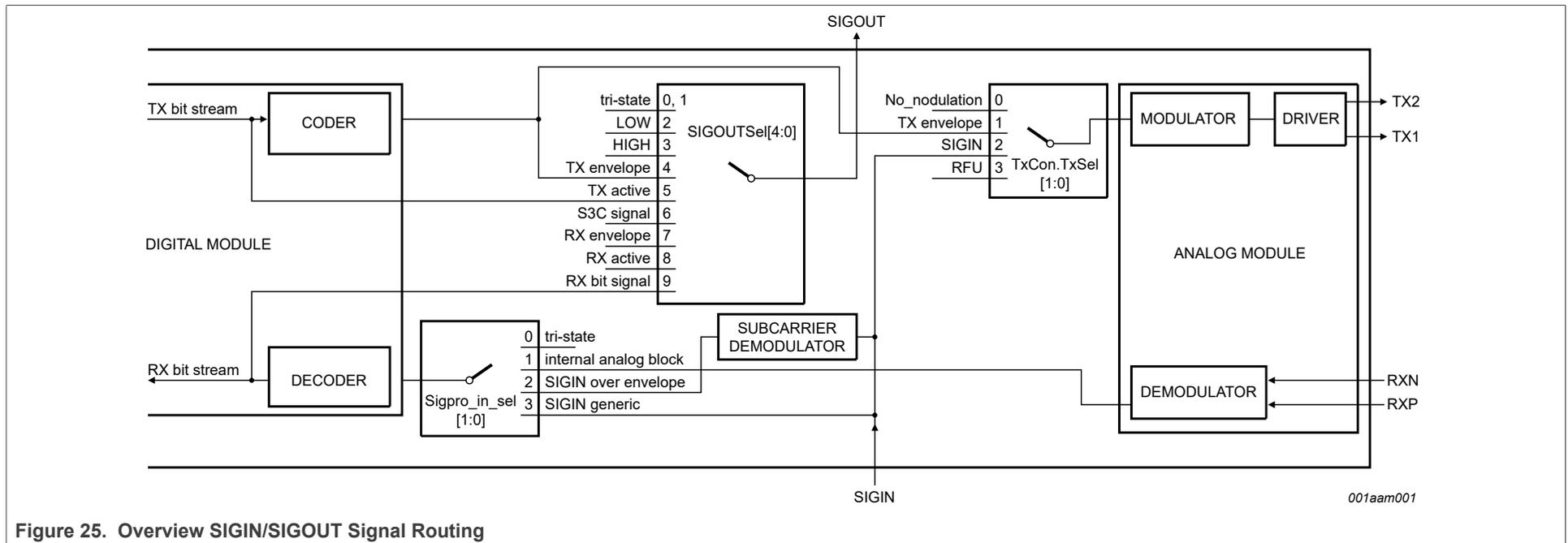
Figure 25. Overview SIGIN/SIGOUT Signal Routing
