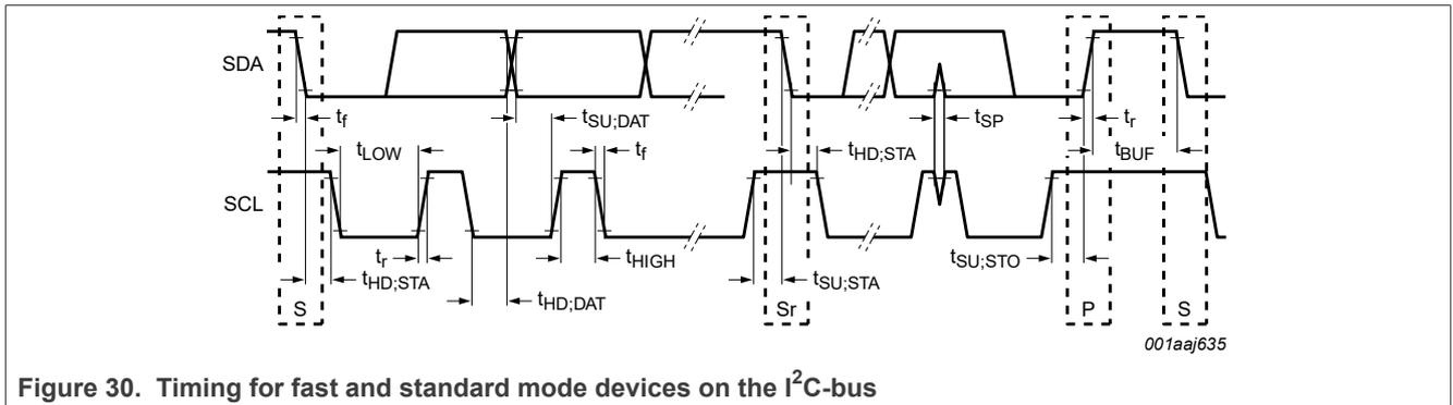
Figure 30. Timing for fast and standard mode devices on the I<sup>2</sup>C-bus
