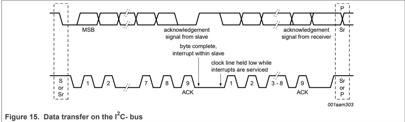
Figure 15. Data transfer on the I<sup>2</sup>C-bus
