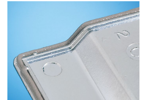
Gasket application to sloped surfaces is fully programmable
