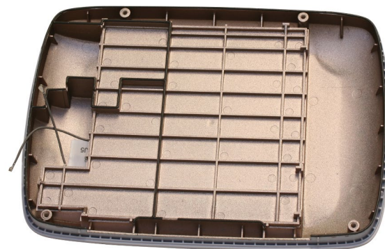
Plastic electronics housing painted with electrically conductive copper-filled coating
