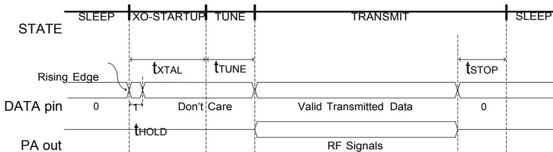
**Figure 16. Transmission Enabled by DATA Pin Rising Edge**
