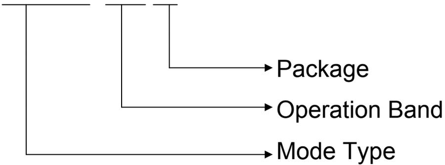
**P/N: RFM119W-315S1****RFM119W module at 315MHz band,SMD Package****P/N: RFM119SW-433S1****RFM119SW module at 433.92MHz band ,SMD Package**
