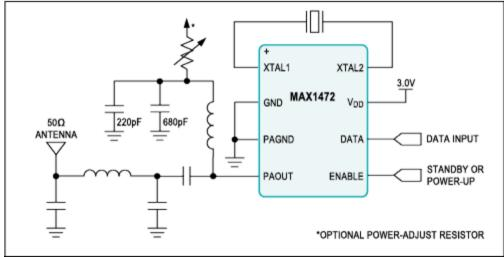
Figure 3. A low-power RF transmitter, based on the MAX1472, delivers a serial data stream using OOK/ASK modulation.
