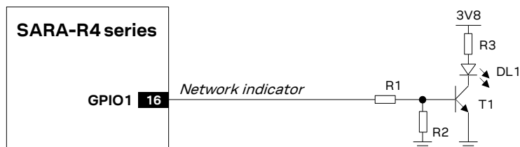
Figure 70: Application circuit for network indication provided over GPIO1
