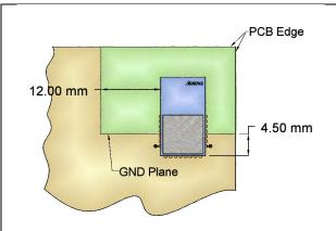
Figure 7 Mounting the module in a corner
