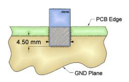
Figure 9 Mounting the module along an edge with overhang. This option is not generally recommended, but is a method to save PCB in an environmentally benign environment
