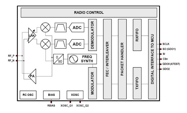
Figure 3 Transceiver IC block diagram.
