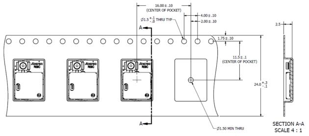
Figure 16 A1101R09C00GR Tape-Reel Packaging Detail (500/Reel)
