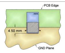
Figure 8 Mounting the module along an edge
