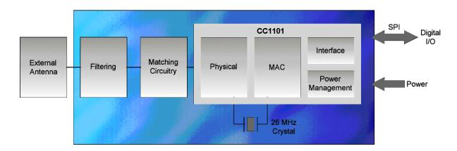
Figure 2 The functionality of the A1101R09C, using an external antenna.
