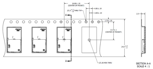
Figure 15 A1101R09A00GR Tape-Reel Packaging Detail (500/Reel)
