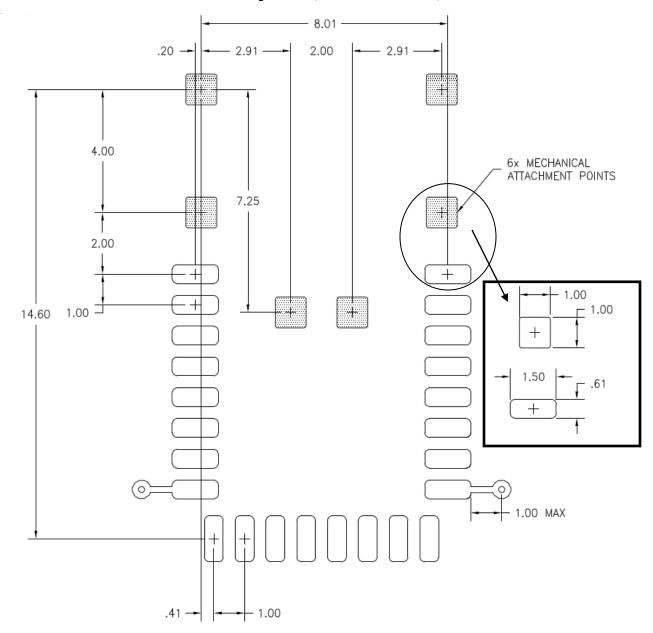
Figure 6 Recommended PCB layout.
