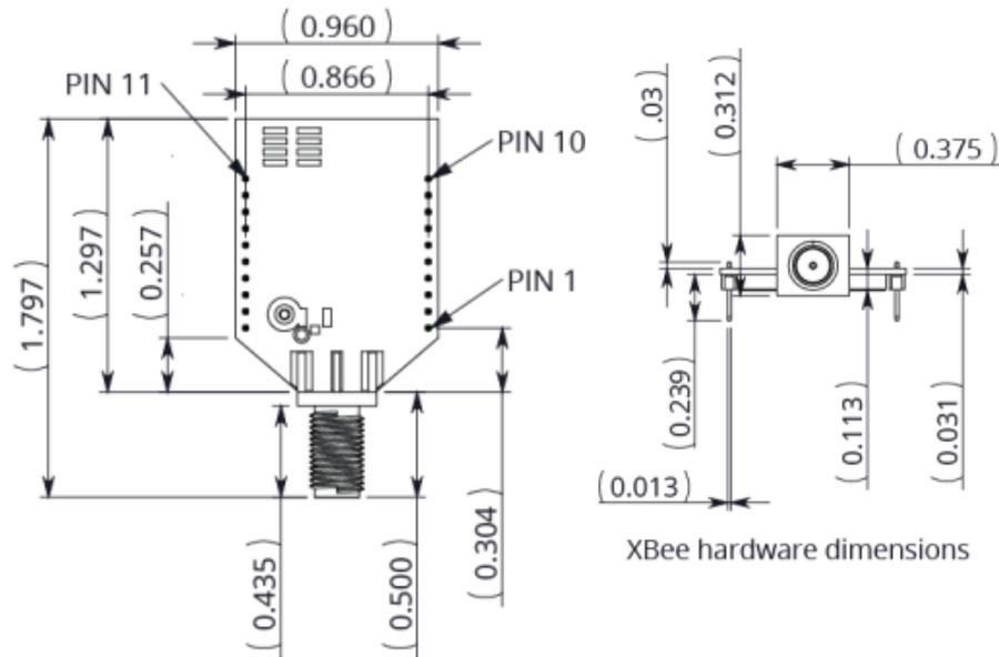
XBee hardware dimensions
