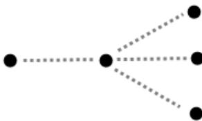
To summarize, the system sends and receives 64 bytes 5 times per second for a throughput of 320 bytes per second with no repeaters and 128 bytes per second with 2 repeaters. Generally, the network throughput decreases by a factor of  $1/(R+1)$ , with R representing the number of repeaters between the source and destination.
