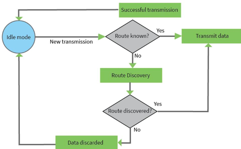
When DigiMesh data is transmitted from one node to another, the destination node transmits a network-level acknowledgment back across the established route to the source node. This acknowledgment packet indicates to the source node that the destination node received the data packet. If the source node does not receive a network acknowledgment, it retransmits the data. For more information, see [Data transmission and routing](#).
