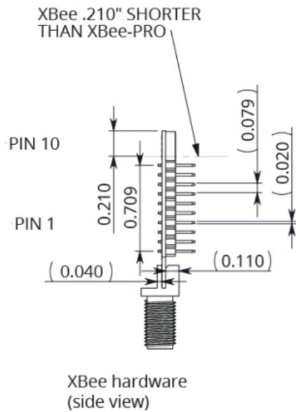
XBee hardware (side view)
