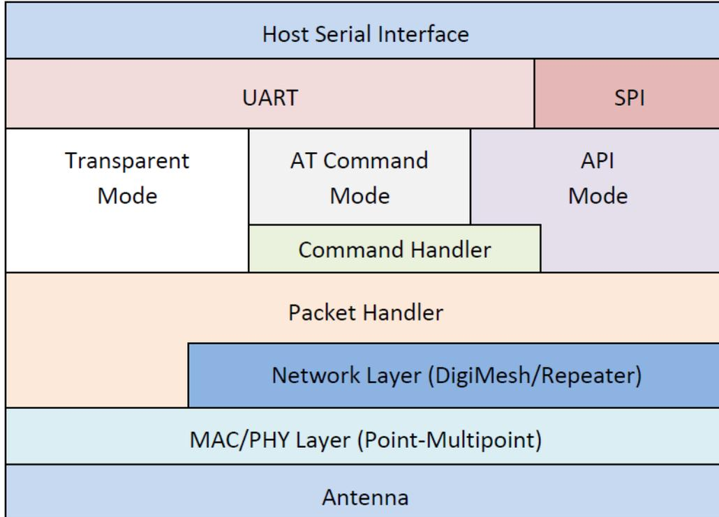
The command handler is the code that processes commands from AT Command Mode or Application Programming Interface (API) Mode—see [AT commands](#). The command handler also processes commands from remote radios—see [Remote AT commands](#).
