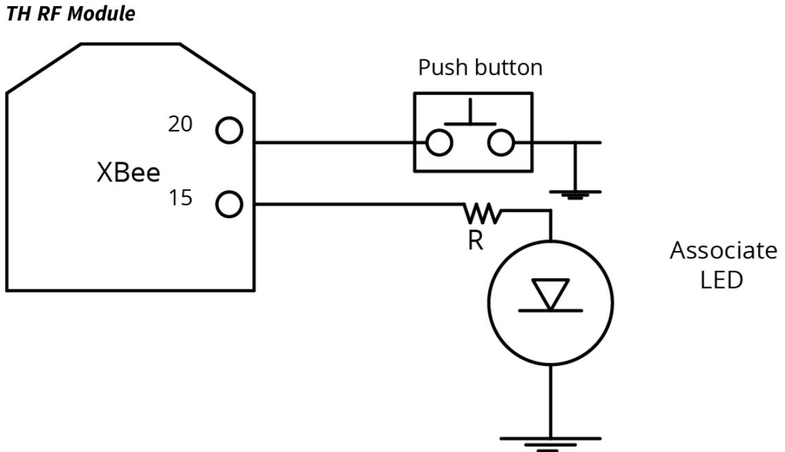
Connect a pushbutton and an LED to XBee-PRO 900HP RF Module pins 20 and 15 respectively to support the commissioning pushbutton and associate LED functionalities.
