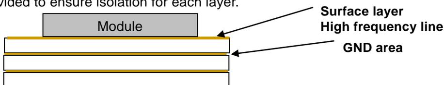
GND pattern of each layer should be connected to GND area with large number of via.
