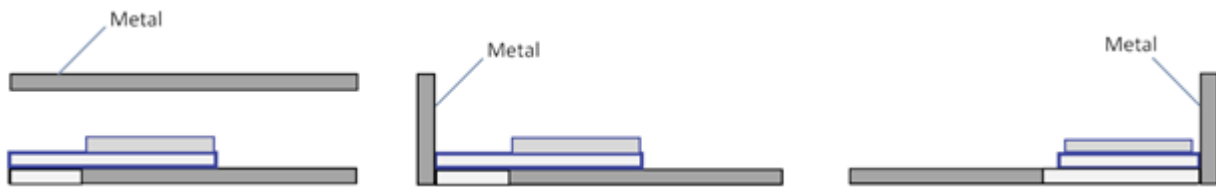
Figure 5-4. Not recommended location in Z plane
