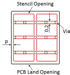
**Figure 14 Stencil Openings Shall not Cover Via Areas If Possible**
