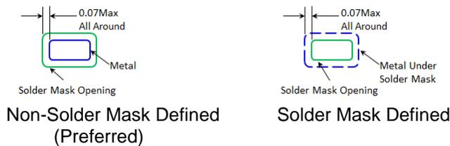
**Figure 11 Solder Mask Pattern**
