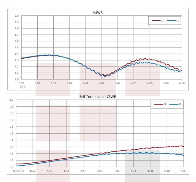
SMA High Power PIN Diode Switch Absorptive From 20 MHz to 6000 MHz Rated at +26 dBm Hot Switching from Fairview Microwave is in-stock and available to ship same-day. All of our RF/microwave products are available off-the-shelf from our ISO 9001:2008 certified facilities in Lewisville, Texas. Fairview Microwave is RF on-demand.
