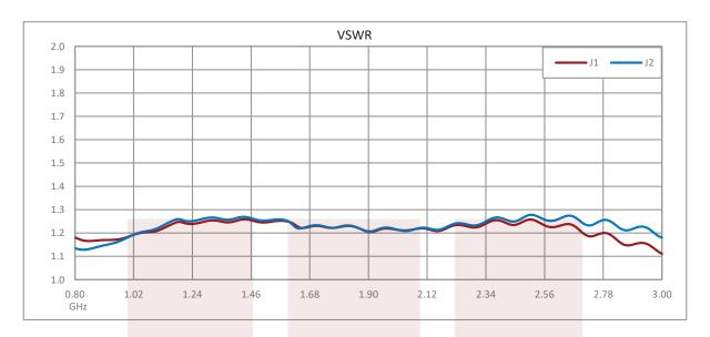
N SPDT High Power PIN Diode Switch From 800 MHz to 3000 MHz Rated at 75 Watts and Hot Switching from Fairview Microwave is in-stock and available to ship same-day. All of our RF/microwave products are available off-the-shelf from our ISO 9001:2008 certified facilities in Lewisville, Texas. Fairview Microwave is RF on-demand.
