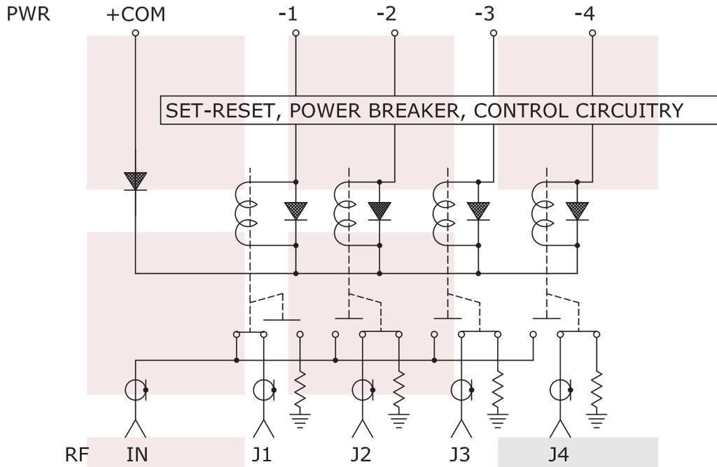
**SCHEMATIC LATCHING WITH 50 OHM TERMINATION
