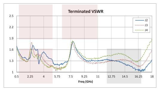
SMA PIN Diode Switch SP3T From 500 MHz to 18 GHz Rated at +20 dBm from Fairview Microwave is in-stock and available to ship same-day. All of our RF/microwave products are available off-the-shelf from our ISO 9001:2008 certified facilities in Lewisville, Texas. Fairview Microwave is RF on-demand.
