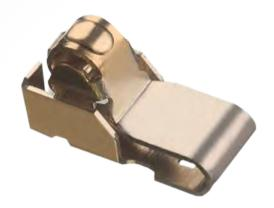
A further development of the extended C style, these contacts were originally designed for wireless antenna connections on many mobile devices, such as smartphones, or LED lamp connection and RFID tags. The Positive Stop shoulder prevents the contact from being over-compressed, which can lead to permanent set and a reduction in spring force.
