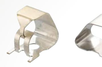
Box style contacts are different to the C style by the addition of a feature that reduces the risk of damage caused by accidental snagging. On some Box designs, it also prevents unwanted lateral movement of the contact during mating. This style can also be labelled as Anti-Hooking.
