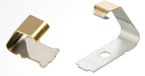
The C style contact is the simplest of designs, providing a flexible connection between PCBs, components and chassis grounds. Manufactured from copper alloy, they provide excellent spring properties over extended periods of time.
