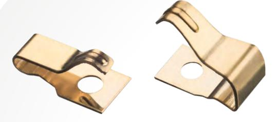
A development of the C style contact, this design uses a more obvious cantilever style. The SMT pick and place area is exaggerated to compensate for the miniature size of the contact. This range is provided in 0.5mm incremental step heights, from 2mm up to 5mm. The footprint is the same across the complete set of contacts.
